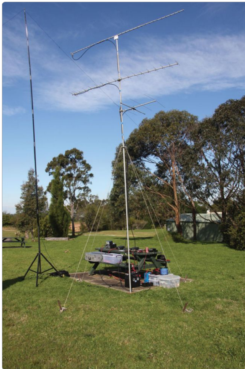
The Manly-Warringah club's VK2MB Field Day station setup at Terrey Hills – 6 m wire antenna held up by the squid pole, with 2 m, 70 cm and 23 cm Yagis on the other mast.
